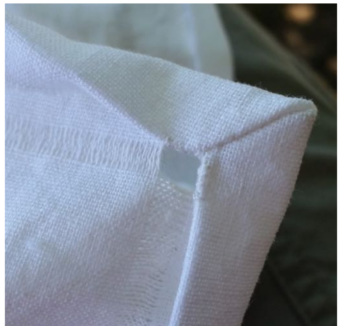
This picture shows the back of a finished mitered corner.
